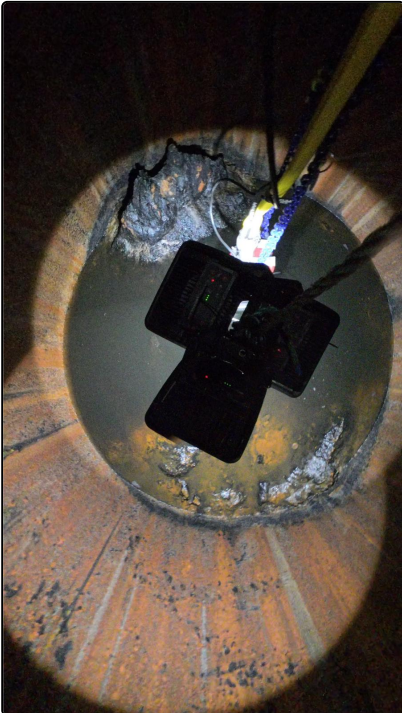
13 Camera and Lights at the bottom of the monopile.
