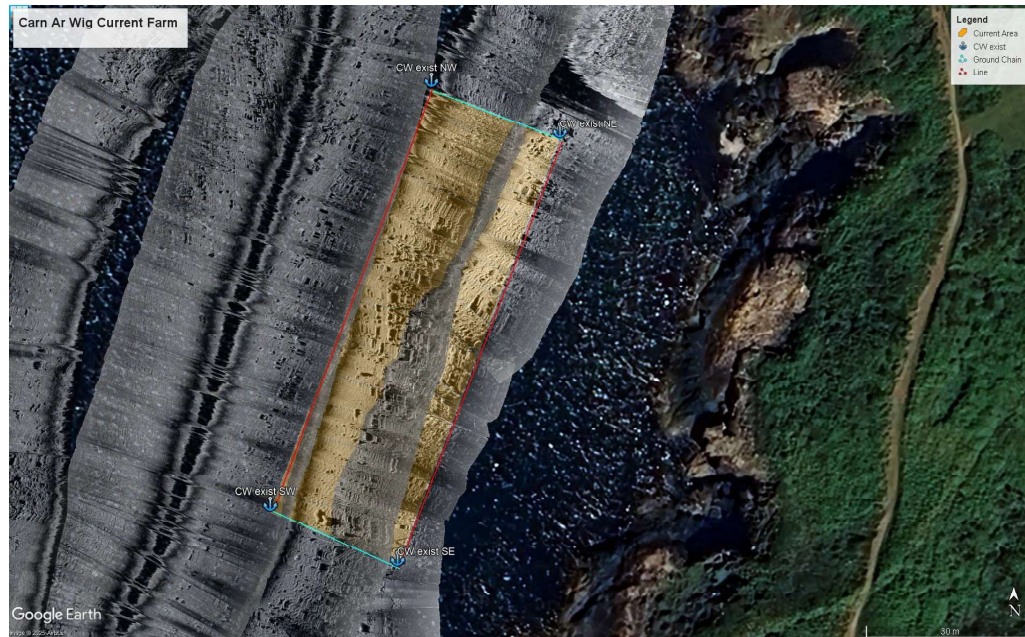
Figure 10. Actual Side-Scan Sonar undertaken at the current Carn Ar Wig site. Red lines represent the current longlines, anchors show the current anchors and blue lines represent the ground chain between anchors.
