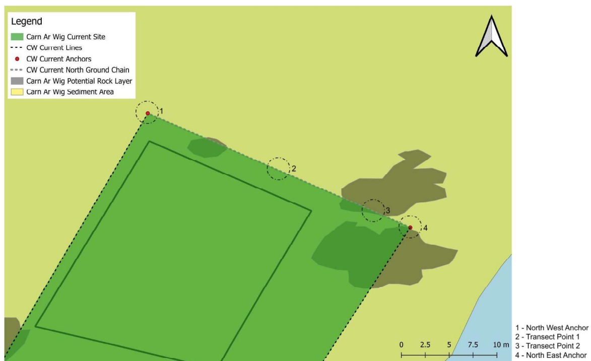
Figure 18. Ground Truthing Points from Diver Footage of the North end of the current Carn Ar Wig farm. Black dotted lines represent the current longlines, red dots show the current anchors and grey dotted lines represent the ground chain between anchors. Yellow areas are sediment and grey areas are potential rocky areas and black circles indicate ground truthing points.
