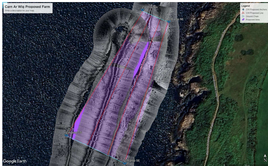
Figure 10. Actual Side-Scan Sonar undertaken at the current Carn Ar Wig site. Red lines represent the current longlines, anchors show the current anchors and blue lines represent the ground chain between anchors.
