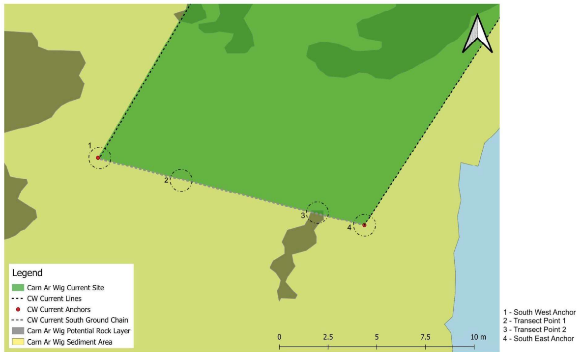
Figure 19. Ground Truthing Points from Diver Footage of the South end of the current Carn Ar Wig farm. Black dotted lines represent the current longlines, red dots show the current anchors and grey dotted lines represent the ground chain between anchors. Yellow areas are sediment and grey areas are potential rocky areas and black circles indicate ground truthing points.
