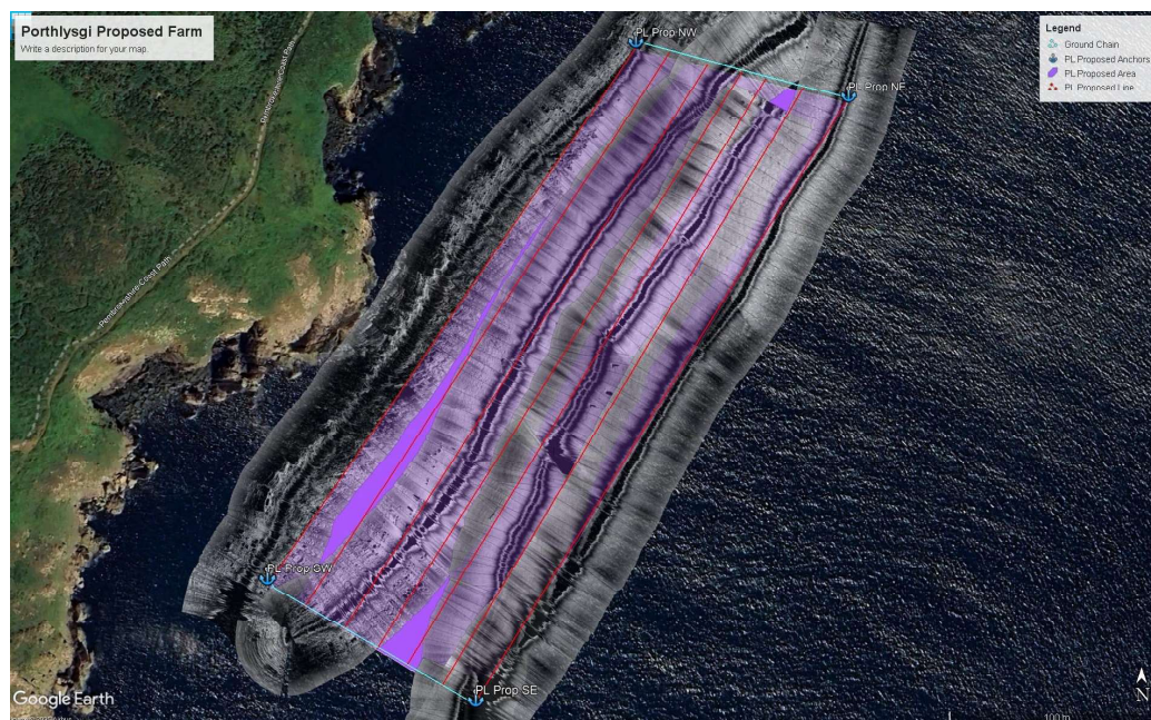
Figure 12. Actual Side-Scan Sonar undertaken at the current Porthlysgi site. Red lines represent the current longlines, anchors show the current anchors and blue lines represent the ground chain between anchors.
