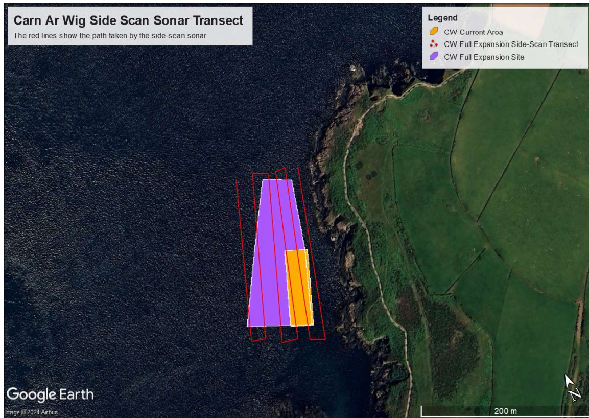
Figure 3. Actual Side-Scan Sonar Transect undertaken at the Carn Ar Wig site. The red continuous line represents the path taken by the Starfish 990F to obtain side-scan data of the seabed across the full expansion site proposed at Carn Ar Wig.
