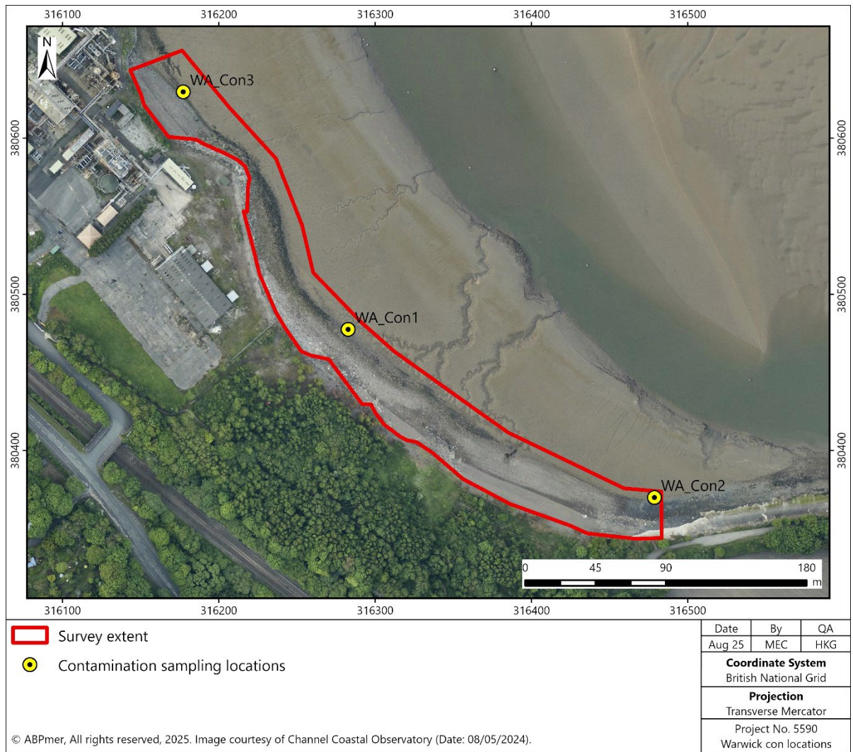
Figure 5. The location of sediment samples collected for contamination analysis at the Warwick site.
