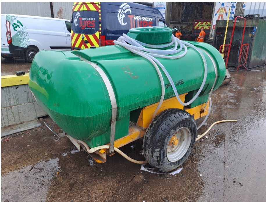
Photo 2 - Water bowser for dust suppression or fire
