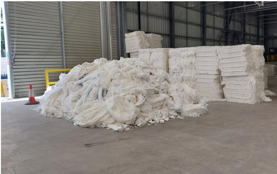
Photograph 1-4: Broke storage and inspection area
