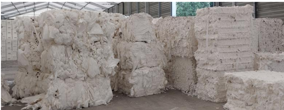
Photograph 1-3: Broke storage bales
