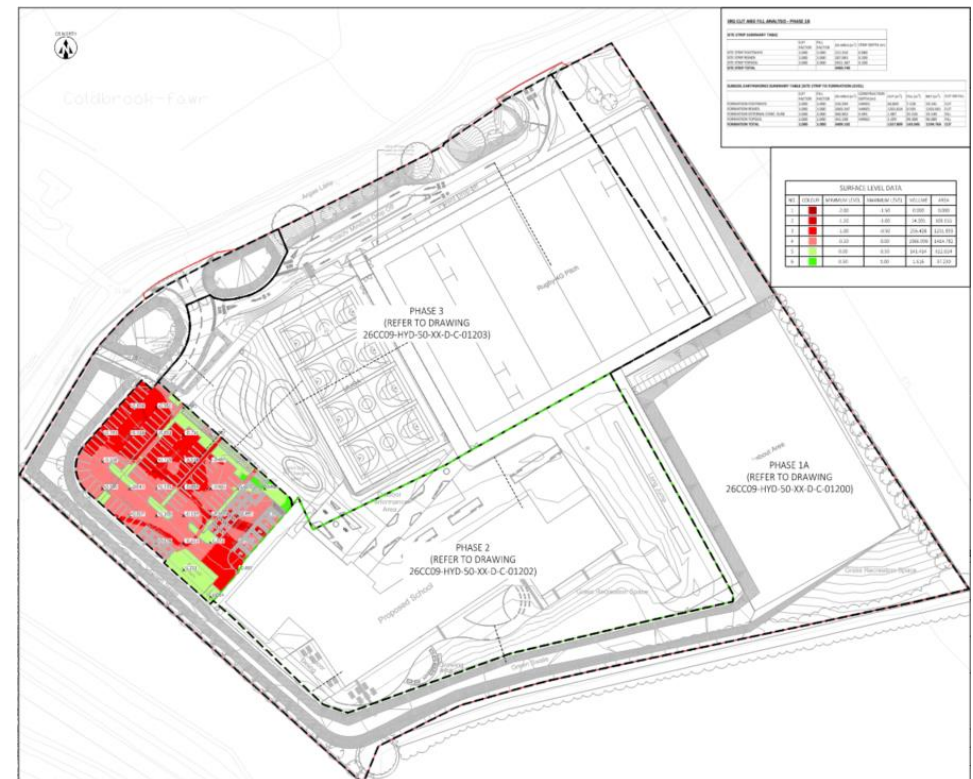
Fig.6.2 – Cut and Fill analysis – Phase 1B
