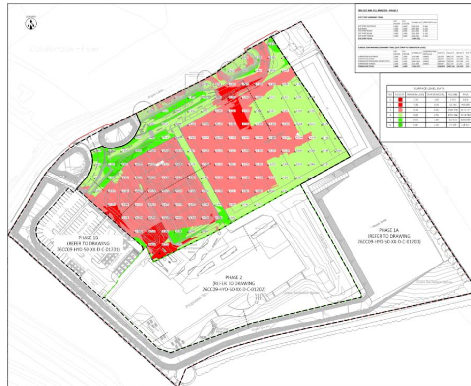
Fig.6.4– Cut and Fill analysis – Phase 3
