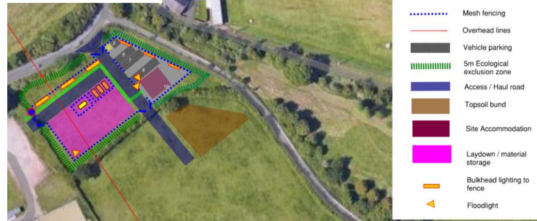
Fig.4.7 – Compound lighting Phase 3
