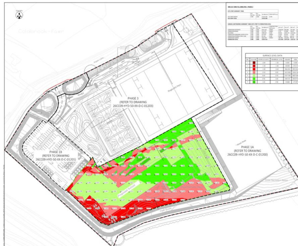
Fig.6.3 – Cut and Fill analysis – Phase 2
