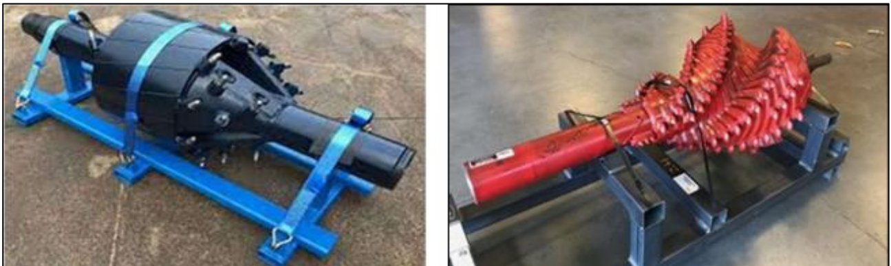
Figure 4.11: Rear reaming assembly
