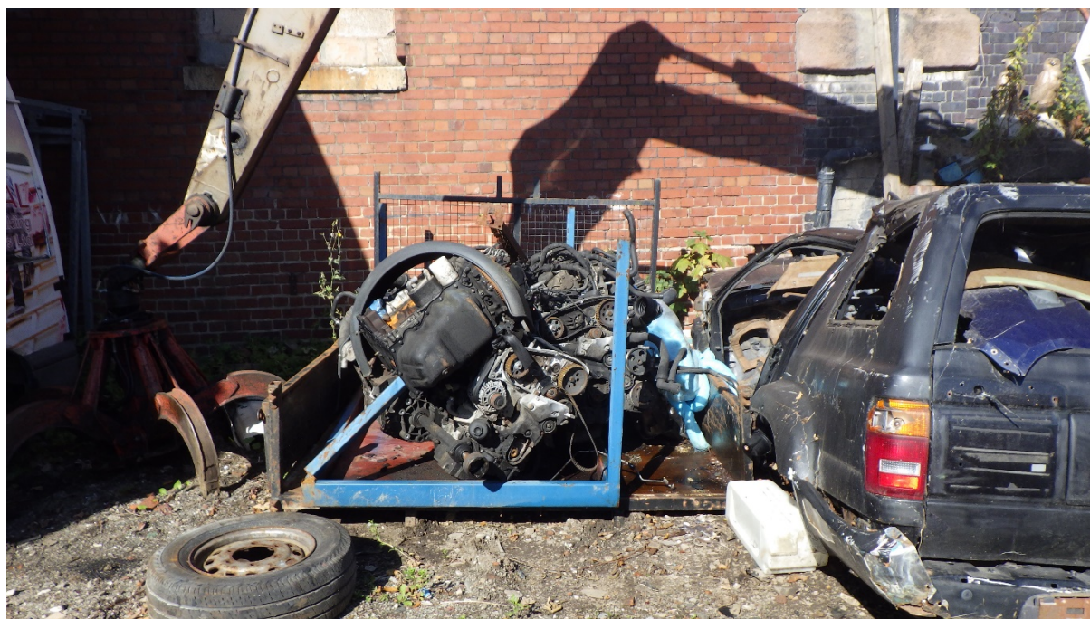
Engines stored in the open on permeable ground
