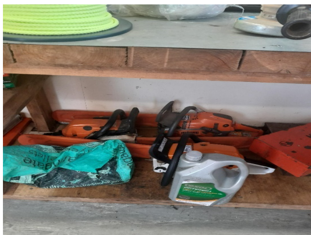
Image 3 – Chainsaws stored outside of bund with oils.
