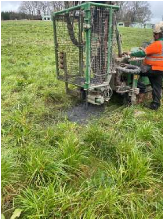
Figure 2-2 BH1 Rotary drilling arisings of Glacial Till
