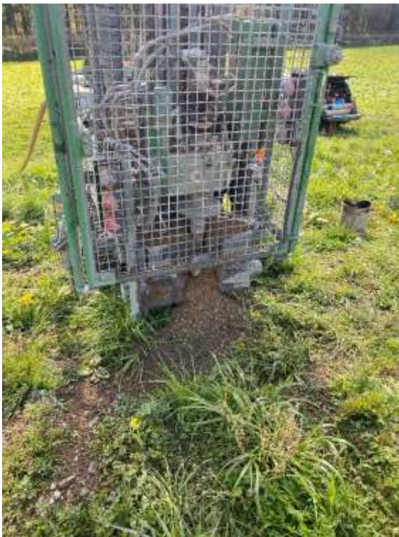
Figure 2-2 BH1 Rotary drilling arisings of Glacial Till
