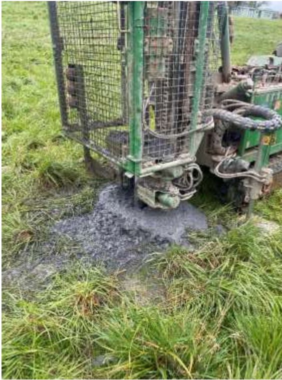
Figure 2-3 Arisings of Laundry Mudstone Formation following water strike
