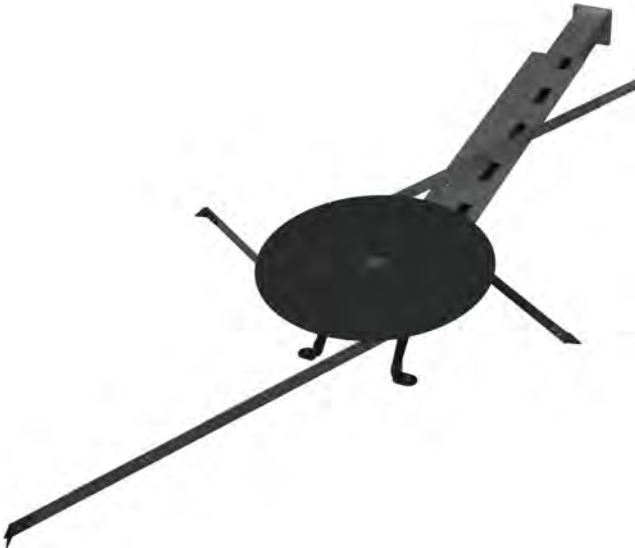
Fig. 12-3: Floor agitator for pellets
