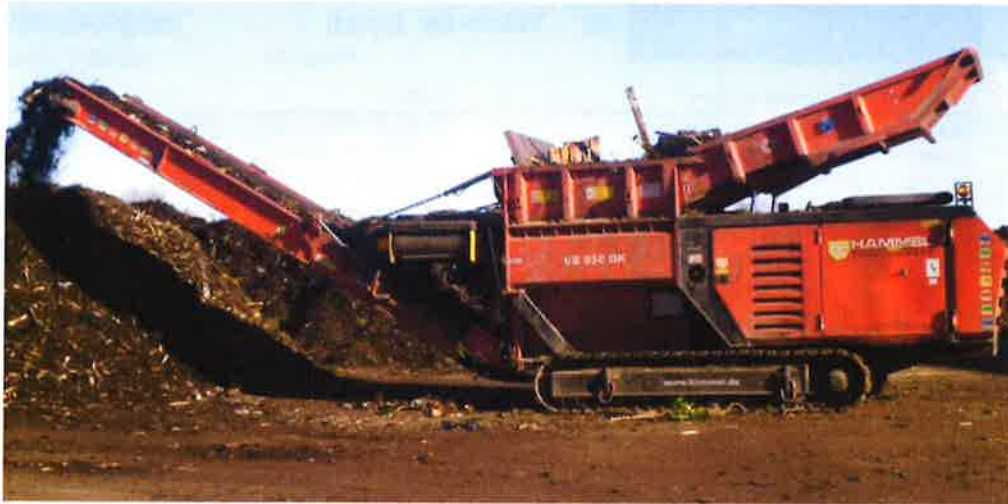
FIG. 4 Wood shredded to form a batch
