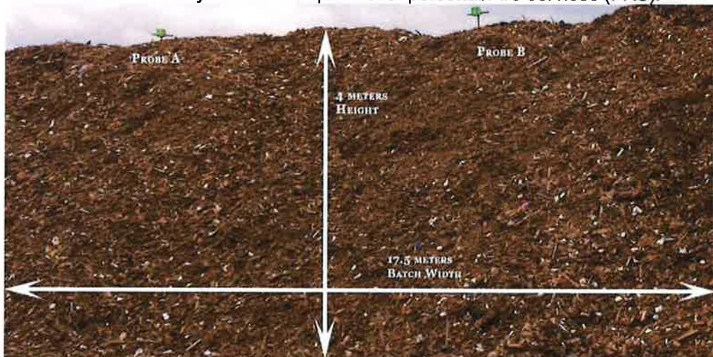
FIG. 7 Shredded Wood Dimensions
