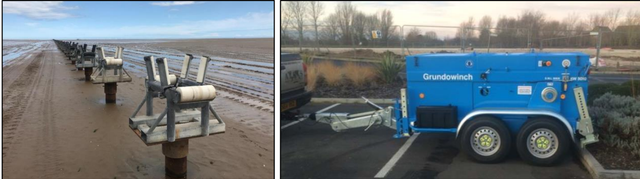
Figure 4.7: Example piled roller highway (left), typical mobile winch (right)
