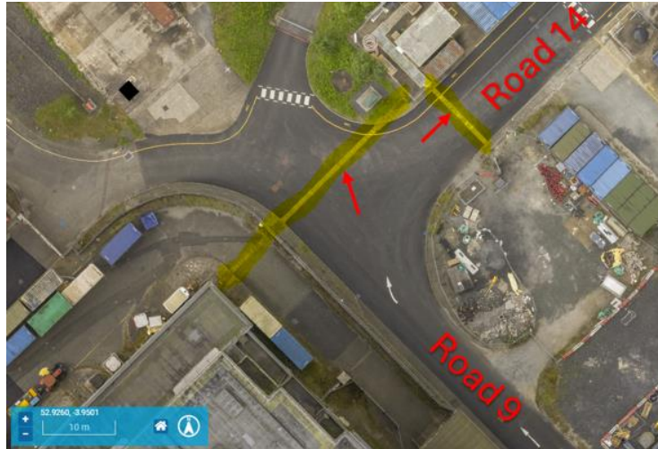
Figure 19 - Aerial view of NE corner of RB2 showing service duct covers
