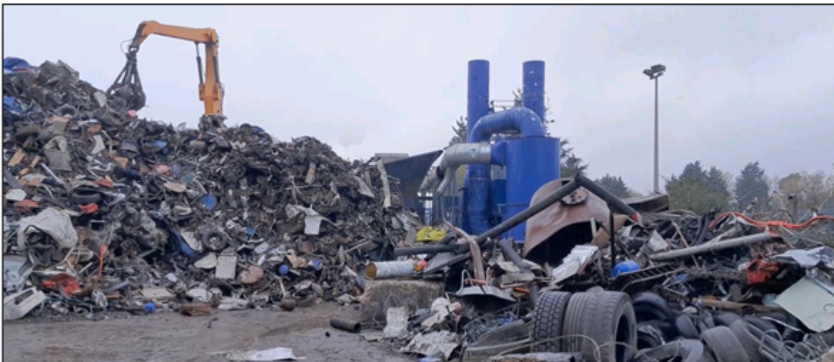
Image 2 - showing the grabber feeding the shredder in use with metal waste
