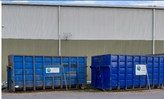
Photo 4. Two roll on roll off skips, one for ferrous, one for nonferrous metals for onward recycling.
