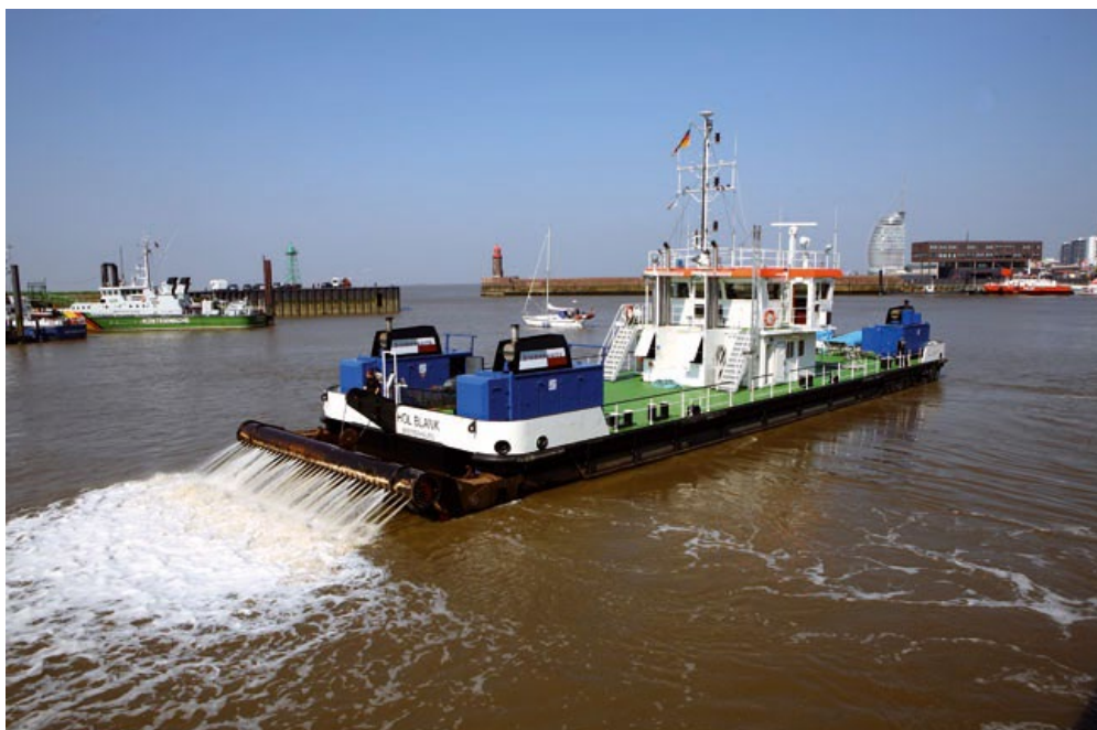
Figure 5 Example of Van Oord's water injection plant
