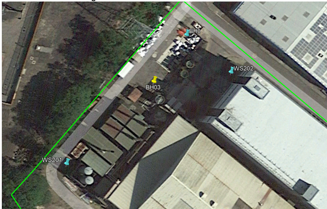
Figure 1: Borehole Location Plan
