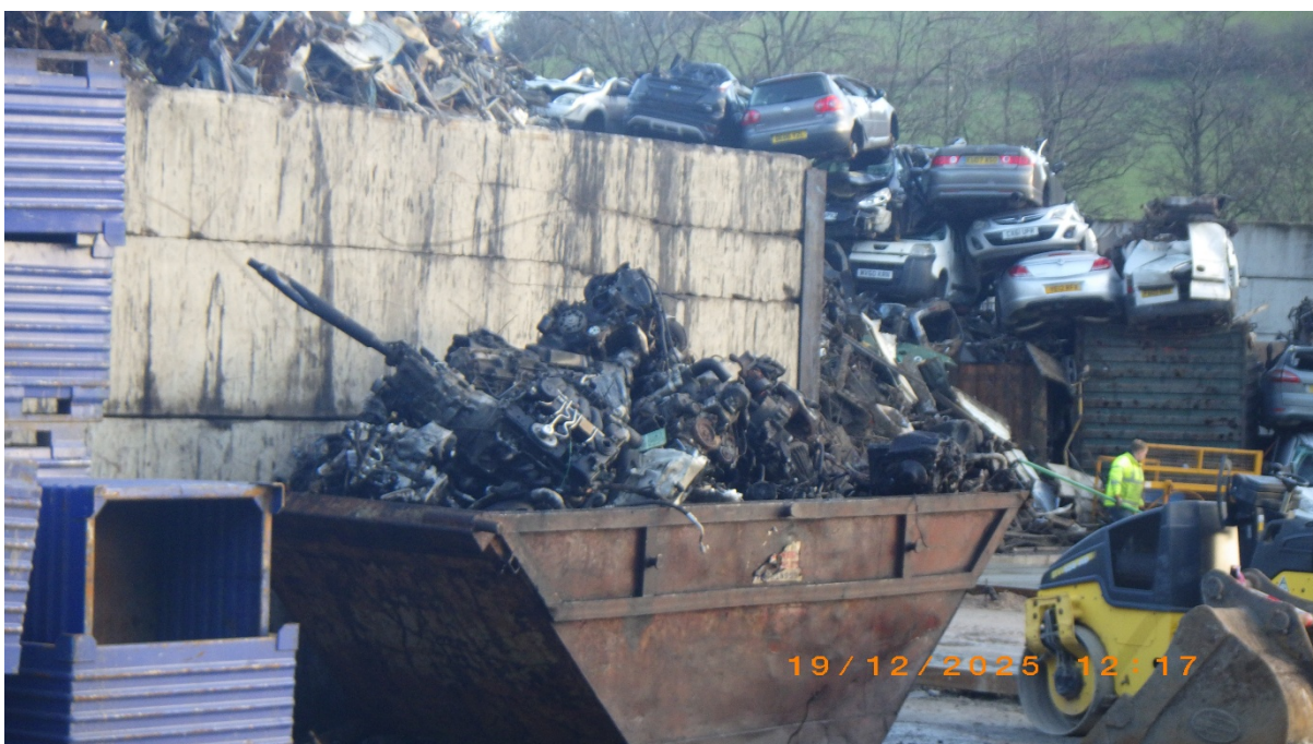
Oils parts stored in an open top skip
