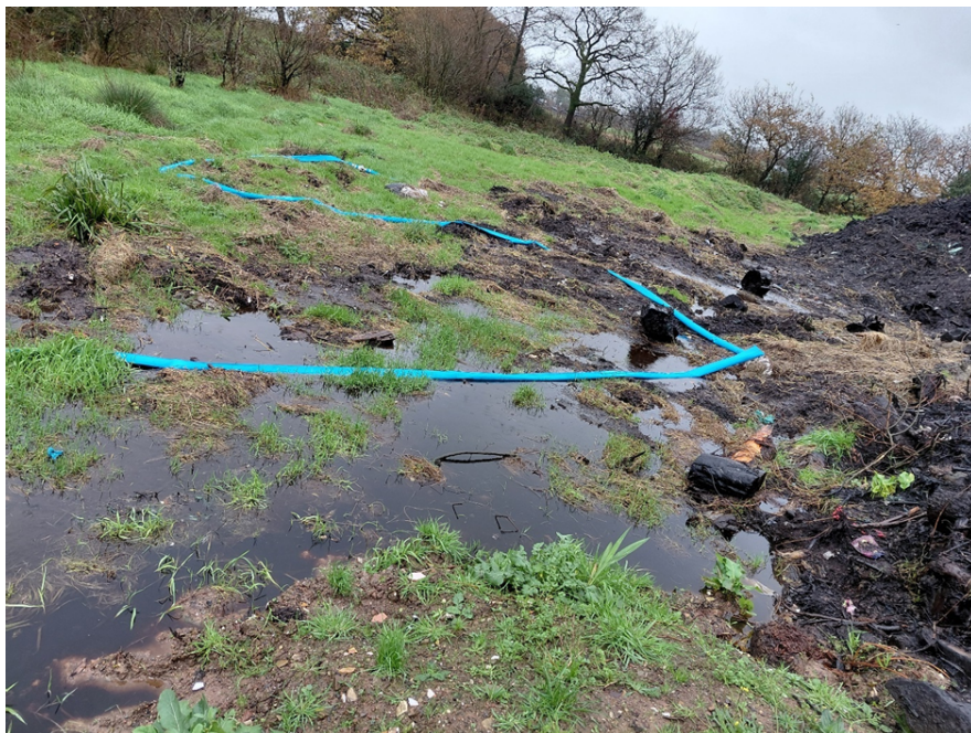
Figure 12 Photo above showing dark brown/black liquid on land adjacent to compost pad.
