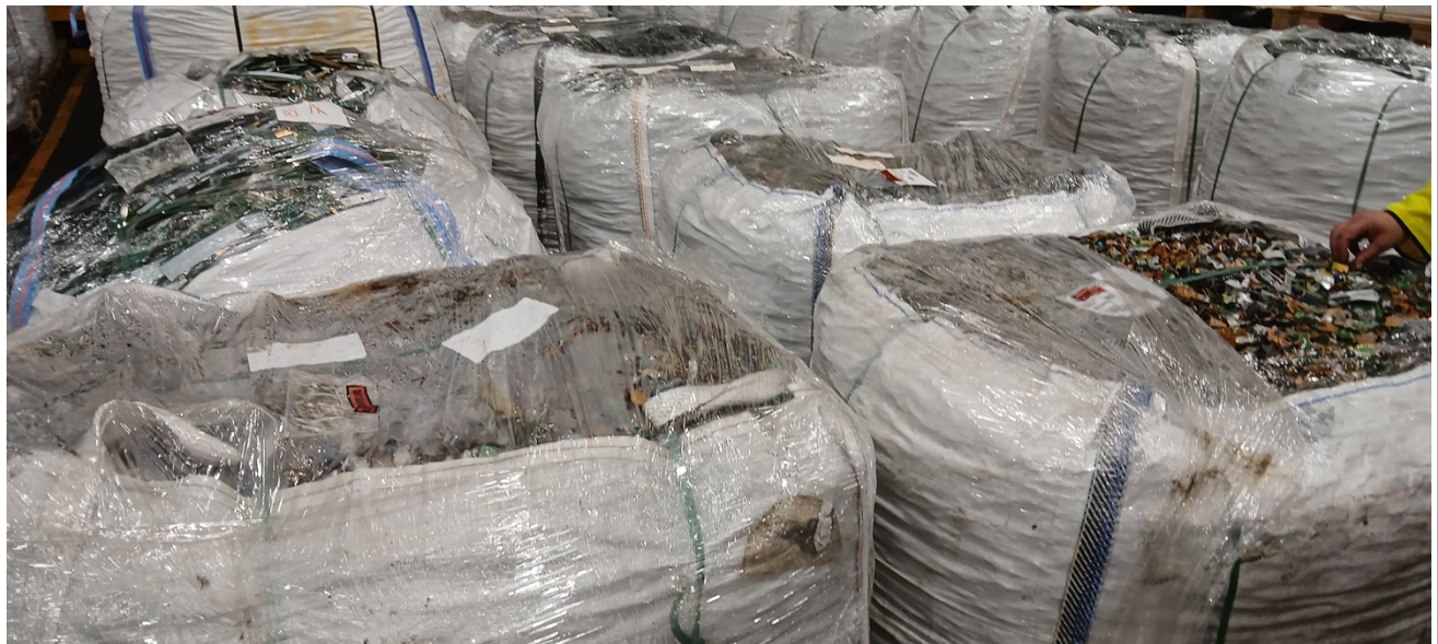
Photo 3 - PCB's ready for the depopulation process within The Royal Mint
