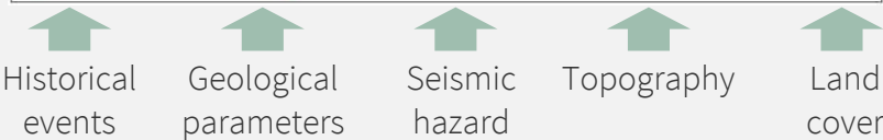
Figure. Input factors considered in the landslide susceptibility index
