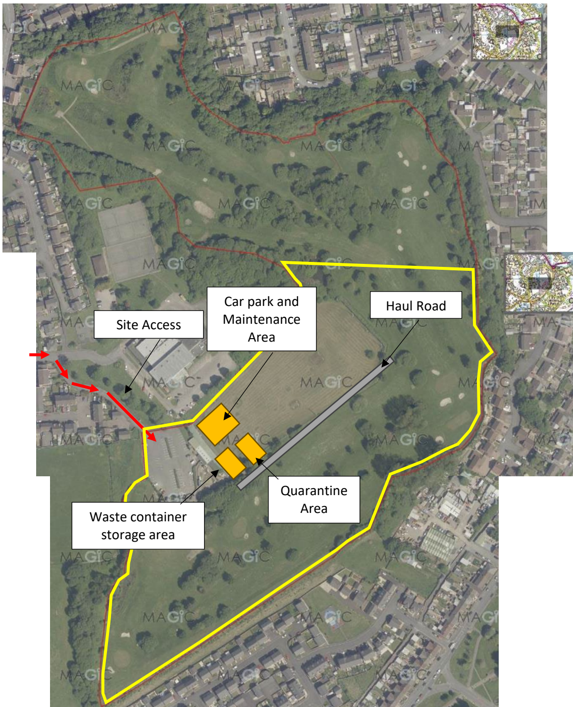
Figure 3: Site access. Note – the haul road location is indicative and will change as the site works progress. There will be no interface between the haul road and the lagoons on site.
