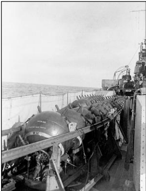
Top right: Horned contact mines on the HMS Aurora .
