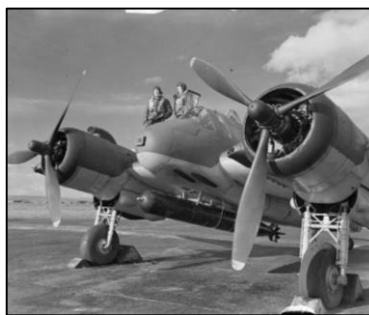
Left: A Mark XII torpedo fitted to a Bristol Beaufighter. Top right: Model of the torpedo. Bottom left: schematics.
