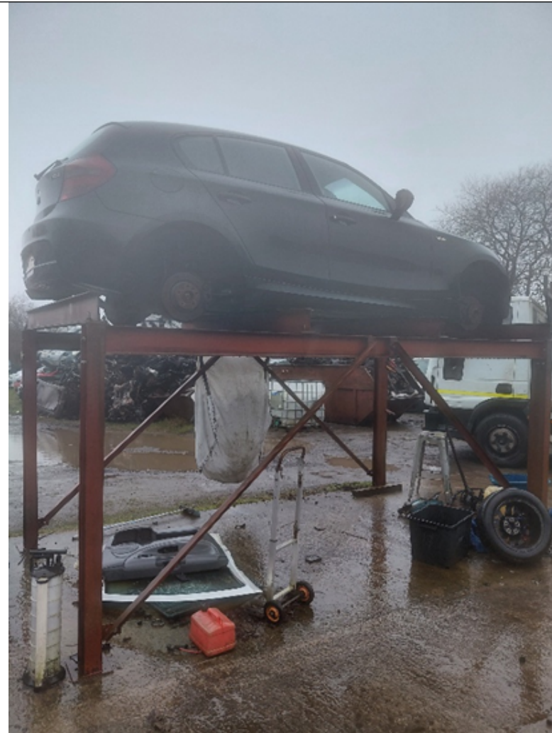
Photo 4. Vehicle on inspection ramps in depollution area.
