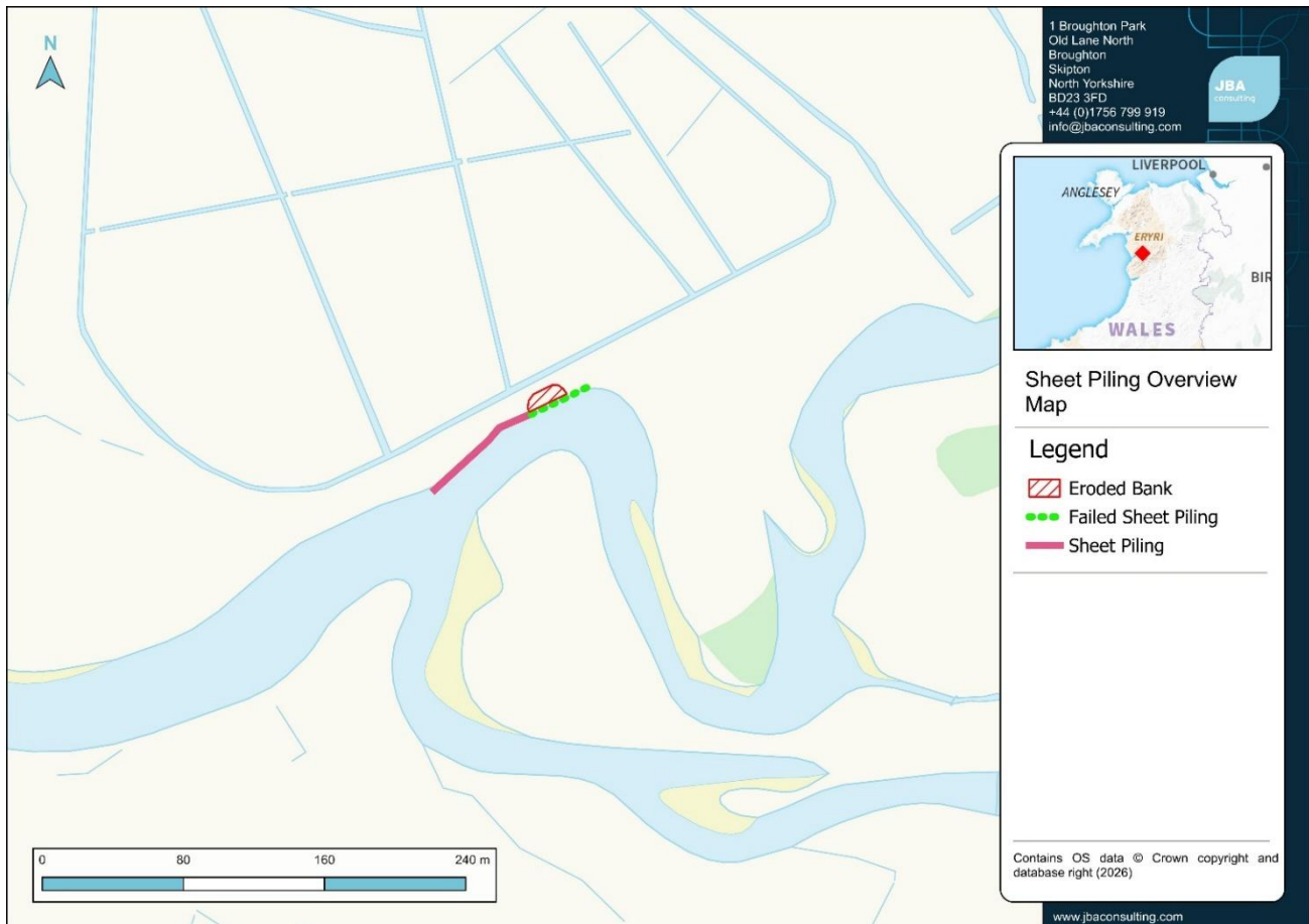
Figure 3-2 Map showing the positioning of the sheet piling, failed sheet piling and area of erosion
