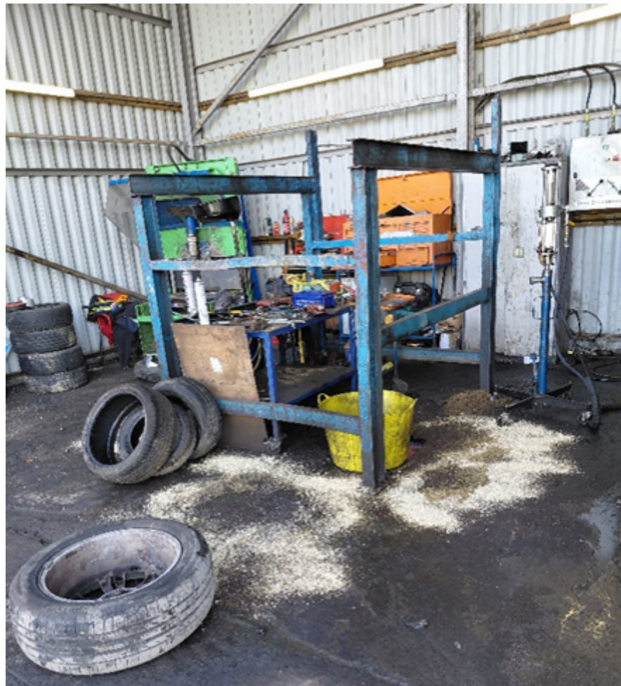
Photo 4. Sawdust being used to contain a small spill
