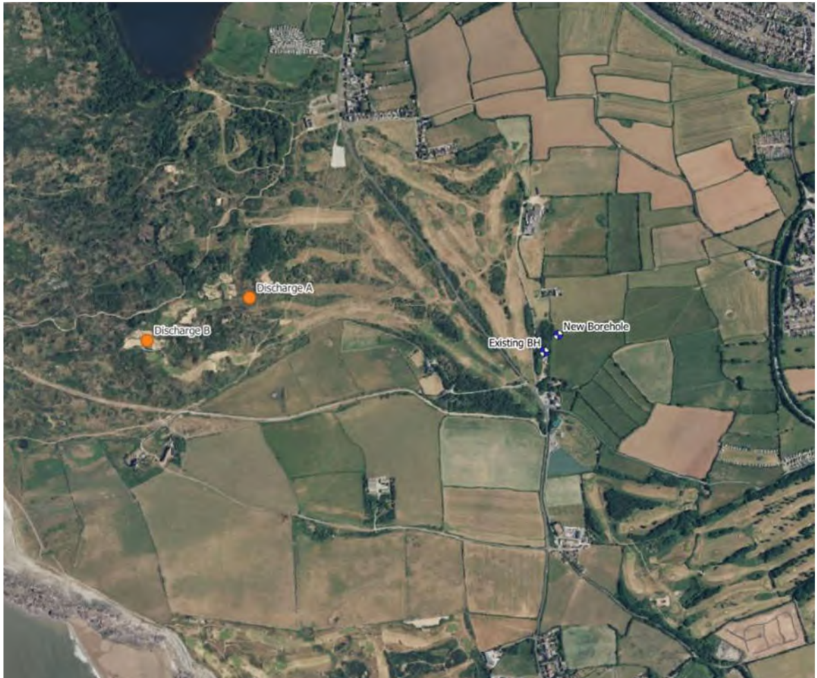
Figure 2-2 Pump Testing Discharge Locations
