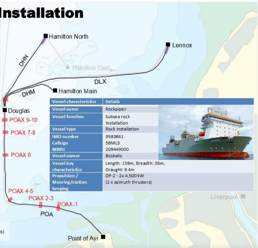
Figure 2-19: Location, and method for post-lay mattress and rock berm installation
