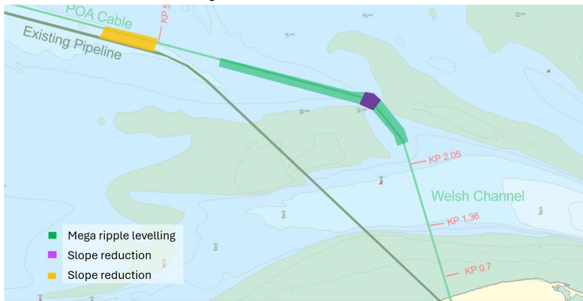
Figure 1 - Execution area of the seabed preparation works based on pre-engineering survey between KP2.000 and KP 5.700
