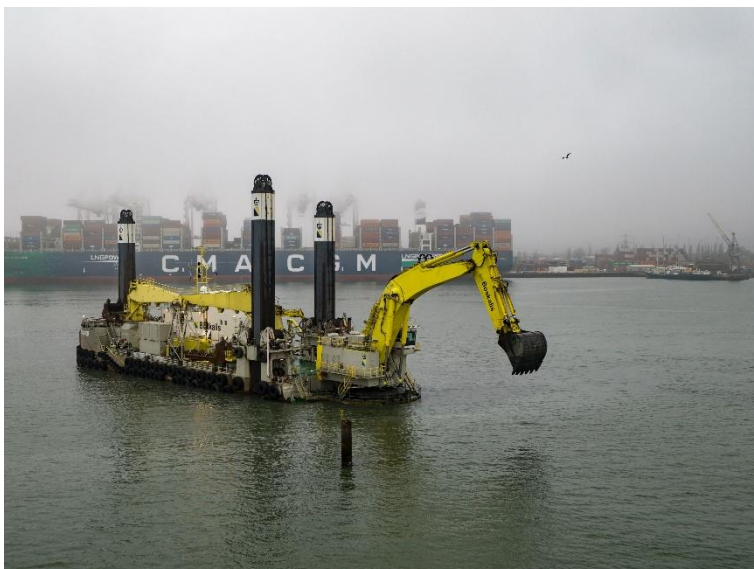
Figure 4 - BHD Magnor side casting configuration
