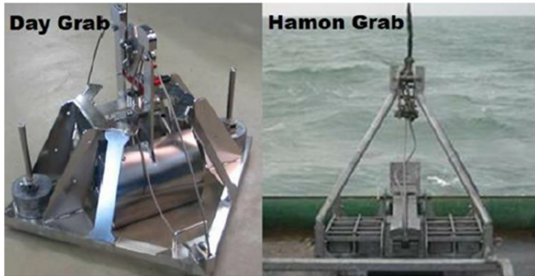
Figure 2.2: Examples of grab samplers
