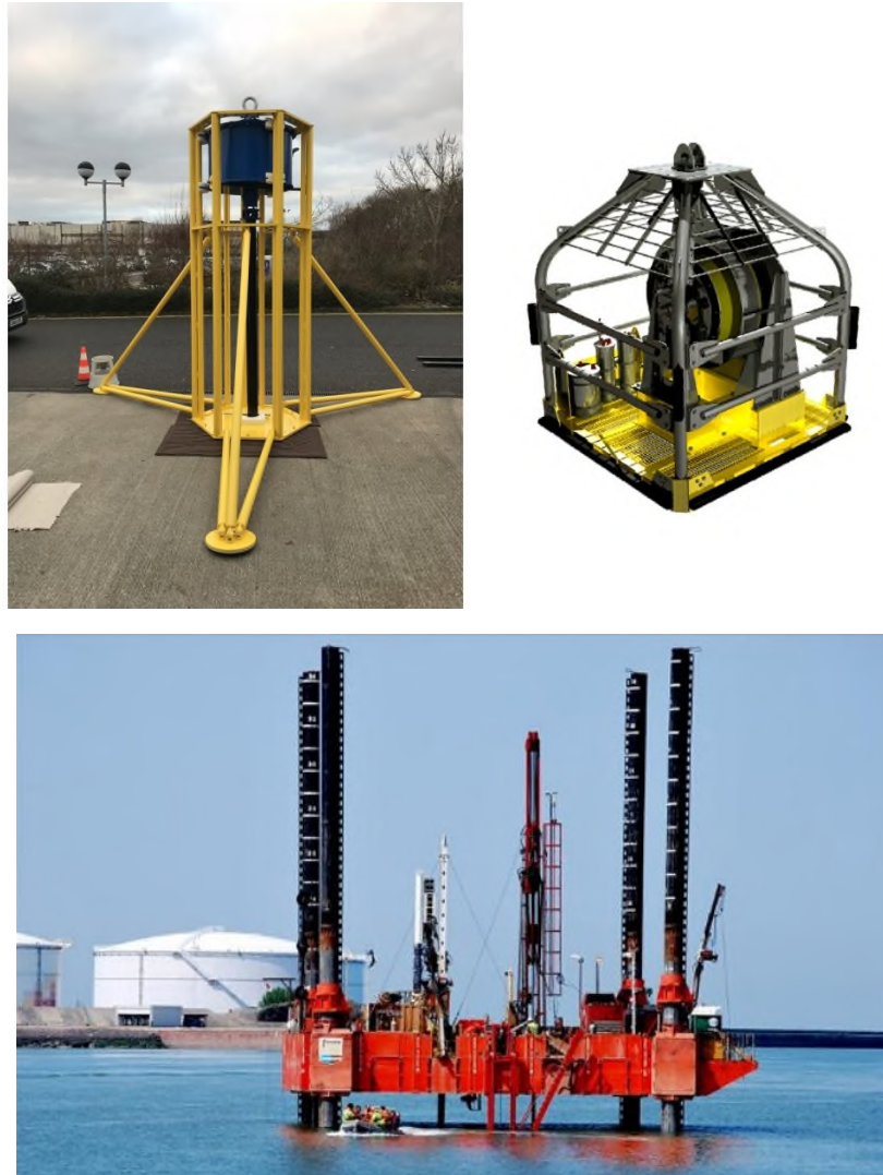
Figure 2.3: Example of a vibrocorer, CPT system, and borehole drilling rig
