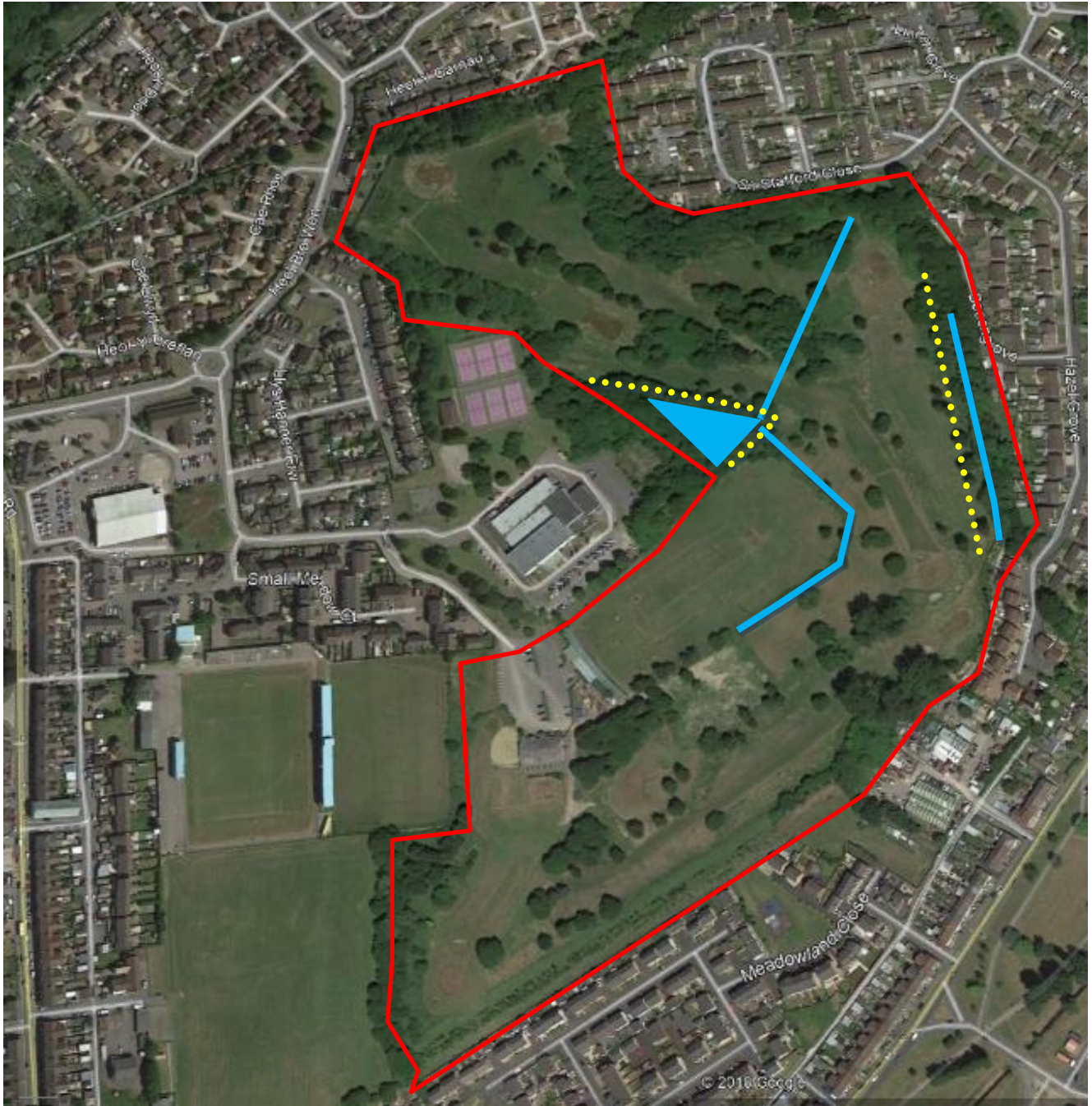
Figure 3: Aerial view of the site showing the locations of the known watercourses on site and protection measures to be put in place.
