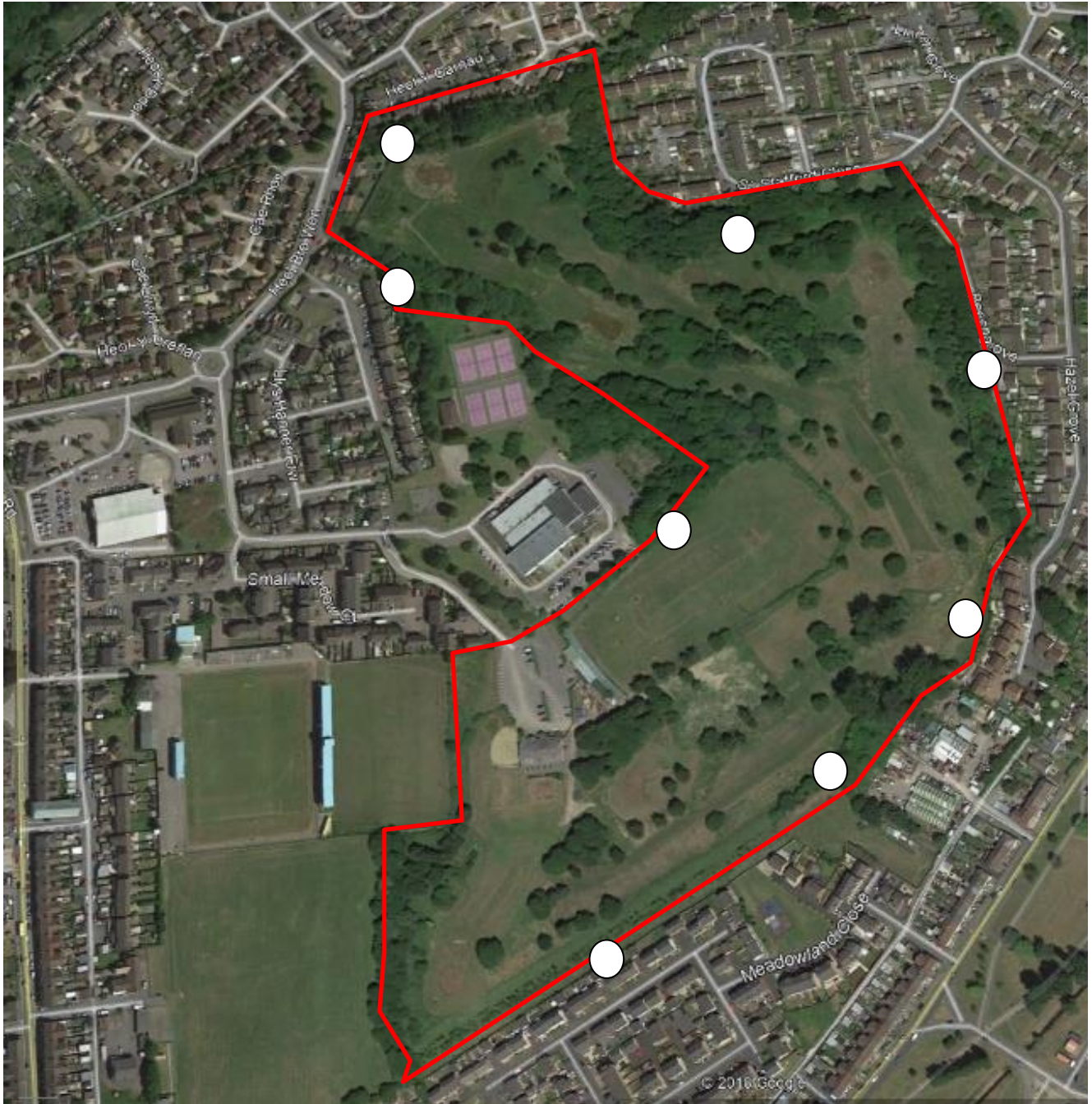
Figure 4: Proposed location of dust monitoring stations throughout the site during the works.
