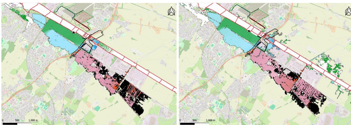
Figure 6.5: 0.5% AEP Tidal 2100 Breach One Flood Depth Difference Figure 6.6: 0.1% AEP Tidal 2100 Breach One Flood Depth Difference
