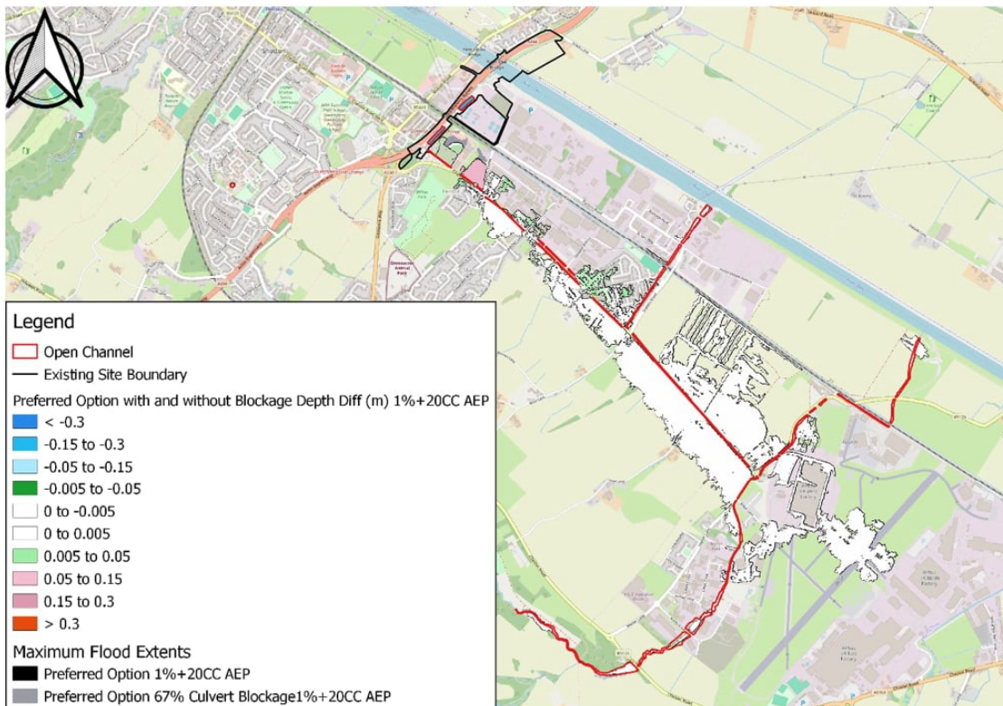
Figure 6.13: Map showing depth difference in the 1% AEP 2100 free flowing and 67% blockage events
