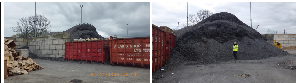
Pile of screened IBA higher than bay dimensions ACTION: Screened IBA pile needs to be reduced in height to be within the dimensions of the designated bay by Friday 22nd May 2026
