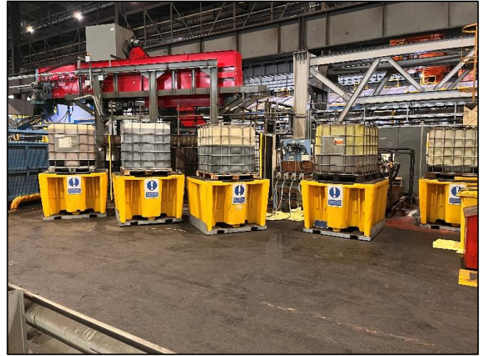
Photographs 1 & 2. Oil storage arrangements at the Automotive Finishing Line (AFL)
