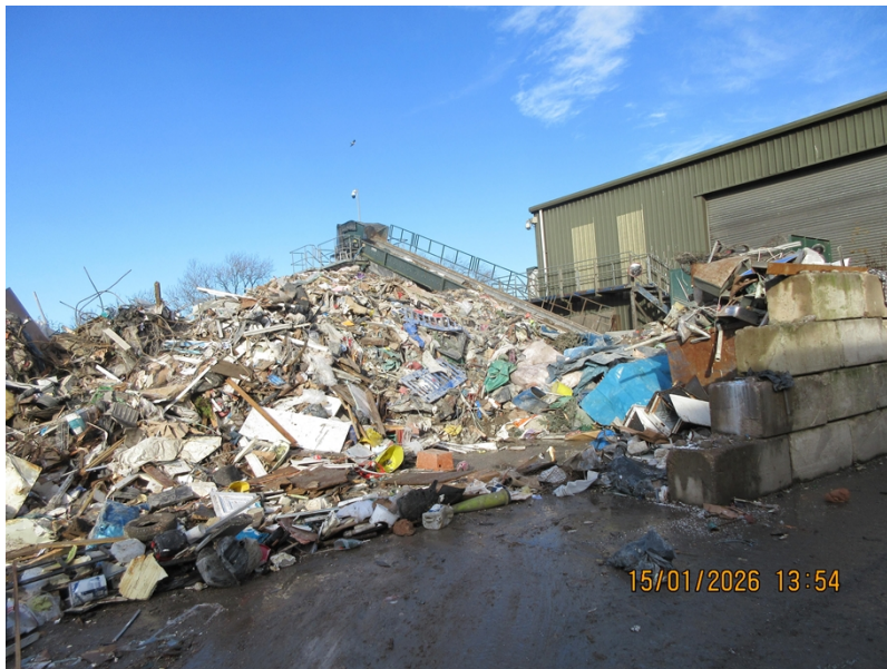
Photograph 1 – Mixed waste stockpile exceeding FPMP recommended height limits.
