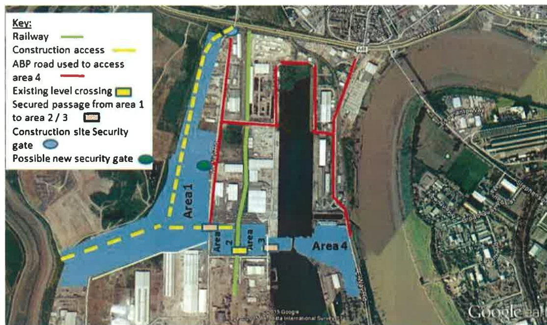
Figure 7c1 – Areas within ABP Newport docks to be used for access and construction of the scheme Source: Buildability Report Update, Appendix SR3.1, December 2016, 6.3.9, figure 6.1
