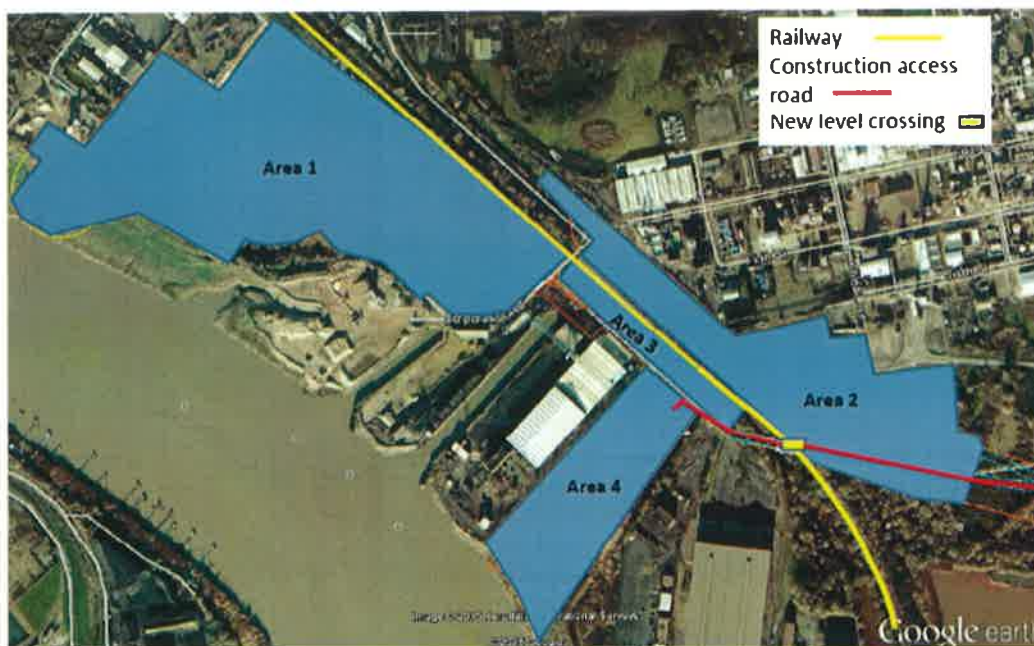
Figure 7c2 – Usk east bank areas to be used for access and construction of the scheme Source: Buildability Report Update, Appendix SR3.1, December 2016, 11.2.1, figure 11.2
