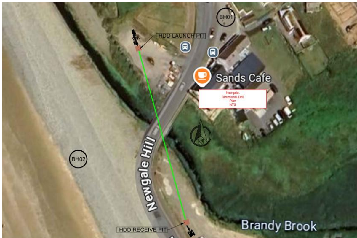
Figure 1-1 Onshore HDD location
