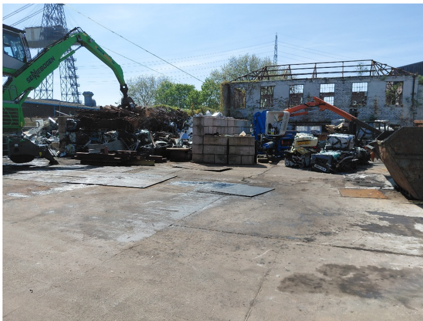
Image 4: Segregation bays being emptied during collection to the left, cubed cars ready for storage to the right.
