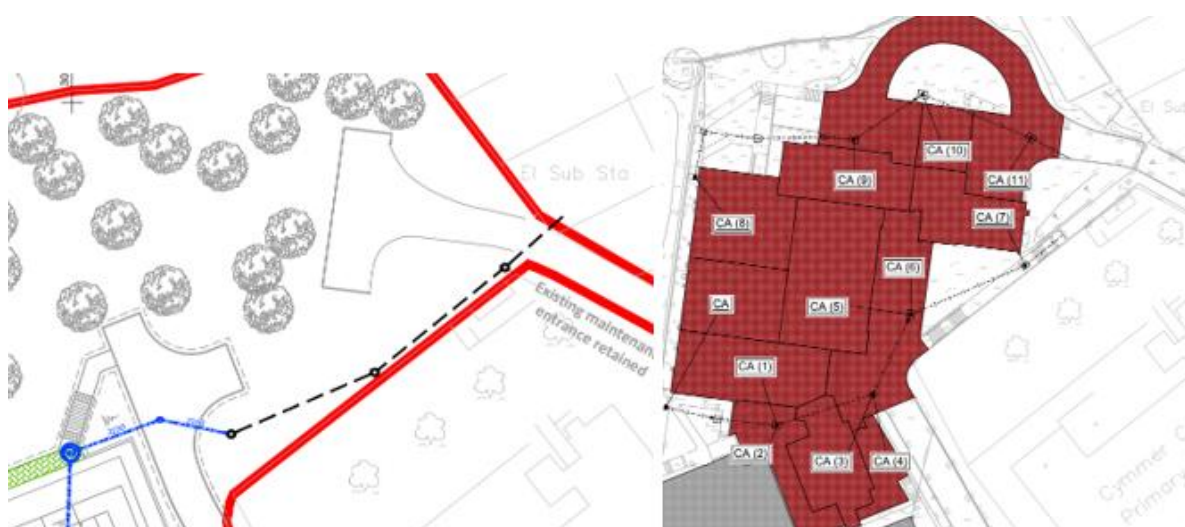
Figure 4. areas that may be included in existing discharge calculation but are to remain freely draining.
