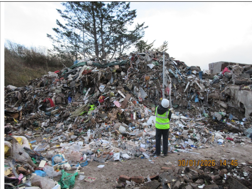
Photograph 4 – Mixed skip waste stockpile exceeding the maximum permitted height of 3 meters.
