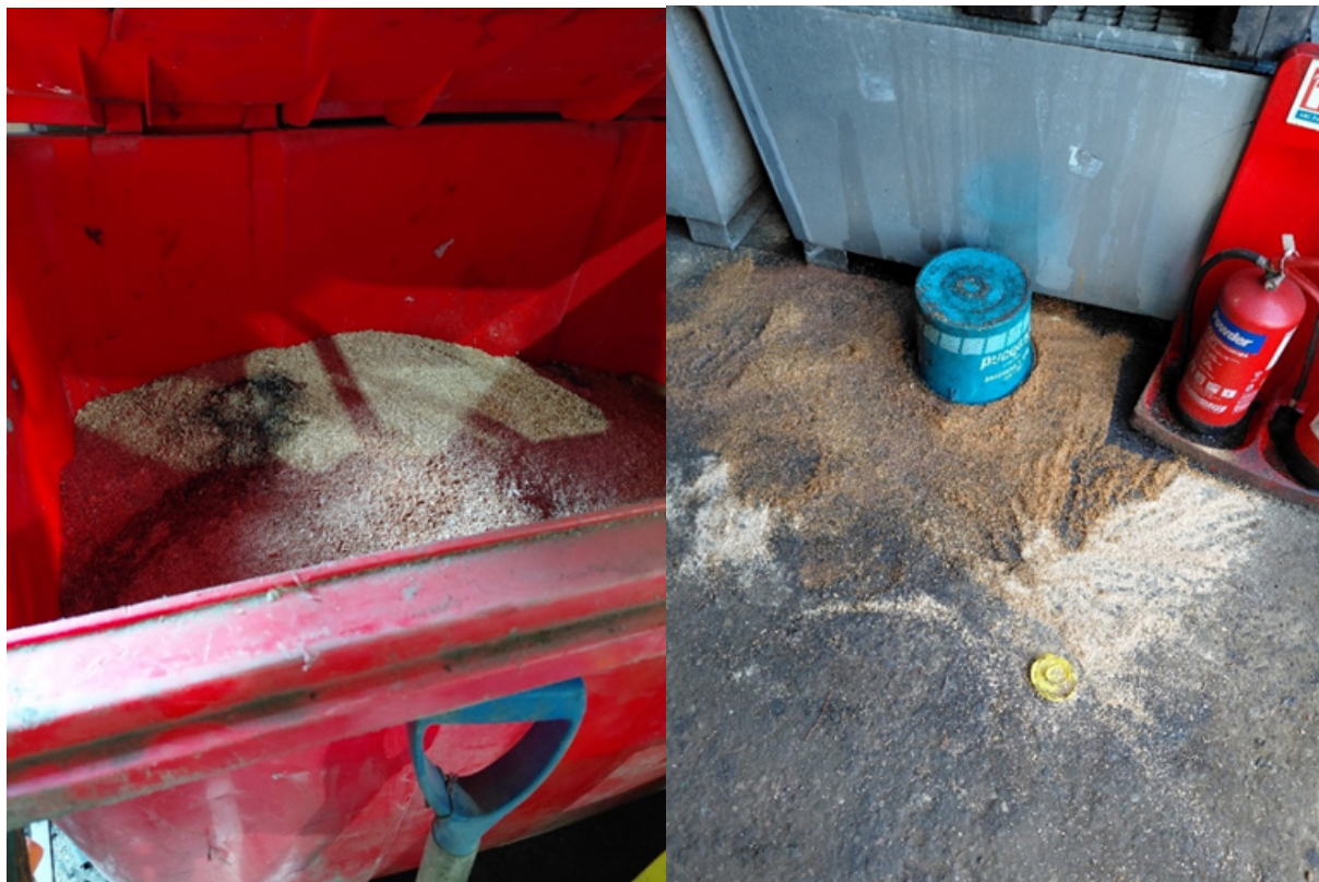
Photographs 4 & 5. Sawdust being used to contain a small spill
