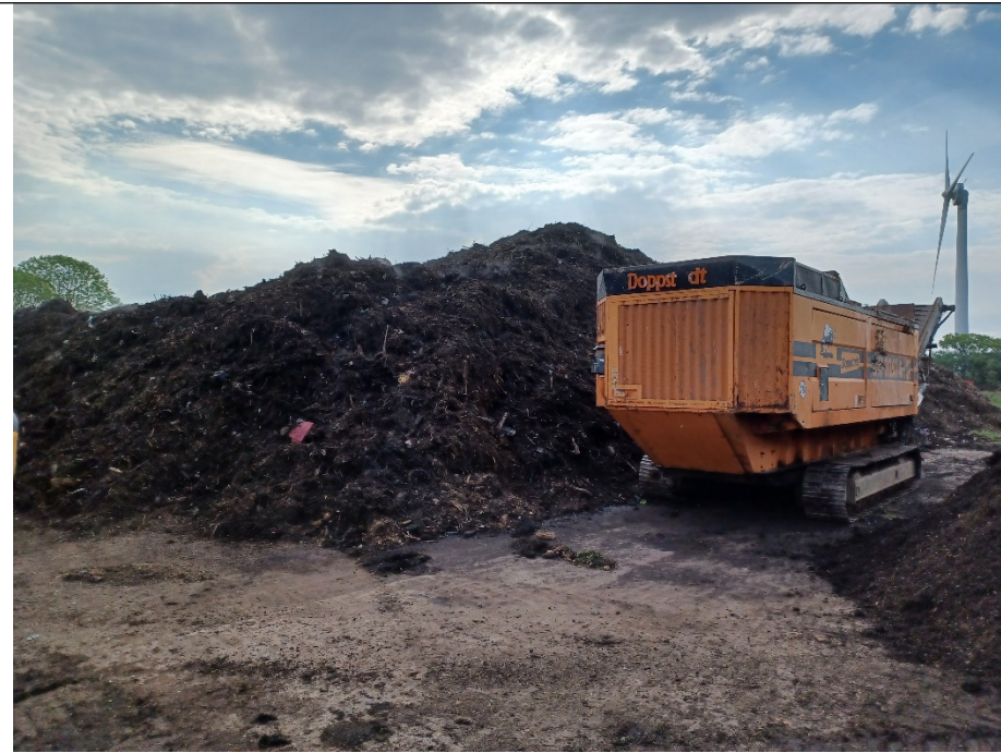
Photo above showing mobile shredder and composting windrows.
