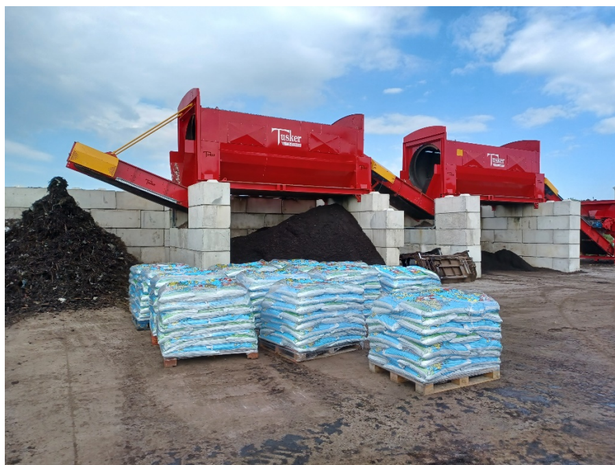
Photo above showing dual drum static screener
