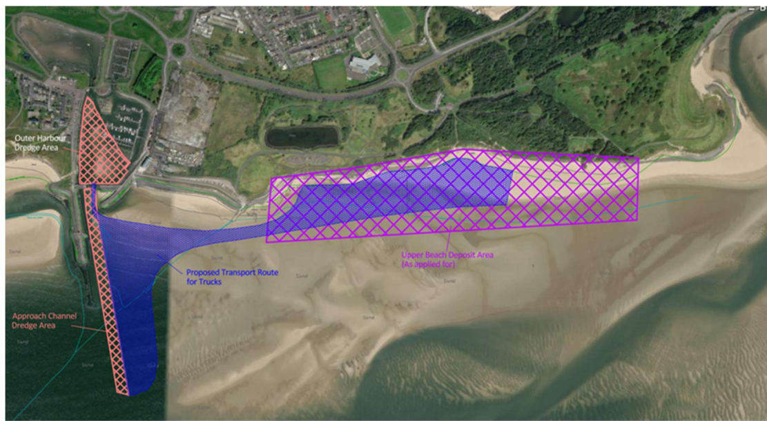
Figure 2 – Dredging and Deposition Locations: Dredging Areas in the Approach Channel and Outer Harbour (orange hatching), Deposit Area on Burry Port East Beach as per the Marine Licence Application (purple hatching), and Transport Area and Deposit Area as per the Dredging Contract Specification (blue hatching)
