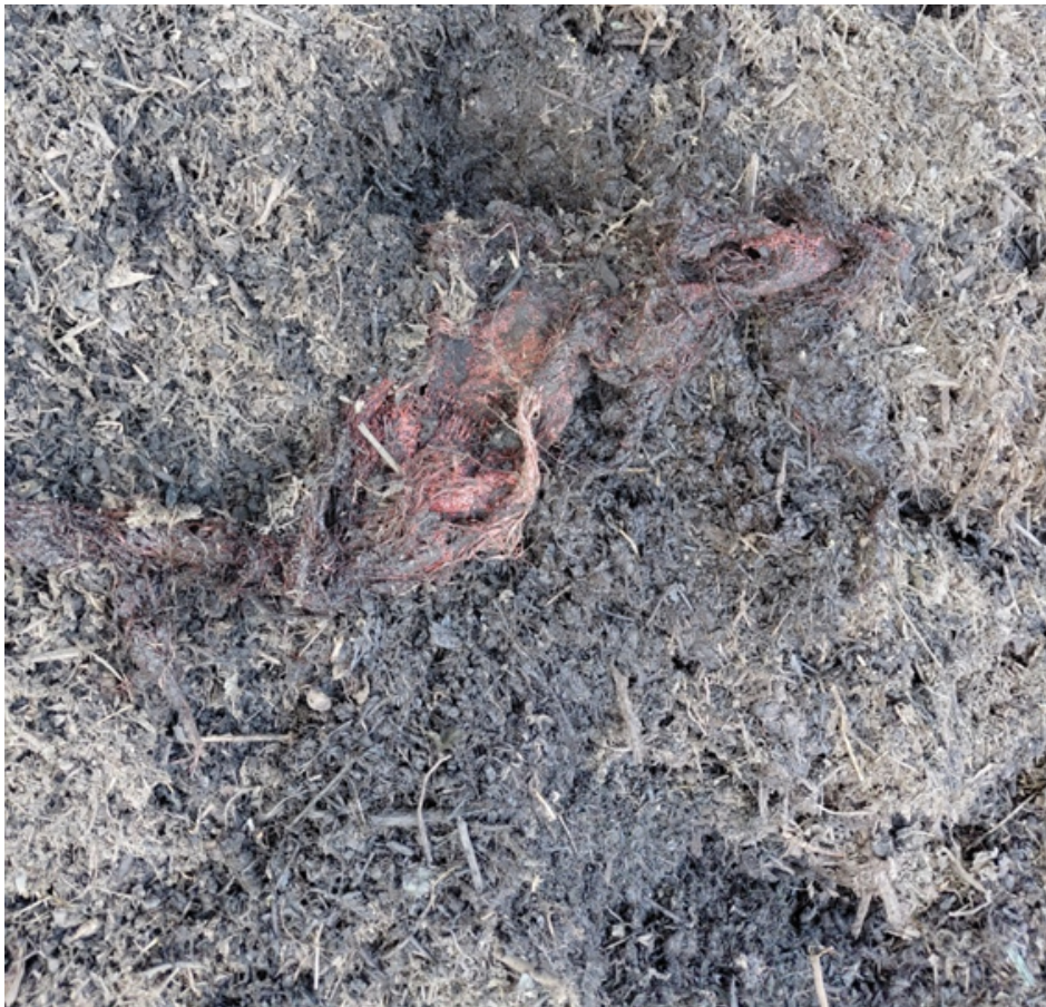
Figure 13 Photo showing contaminants in Batch 358-10 in storage shed.
