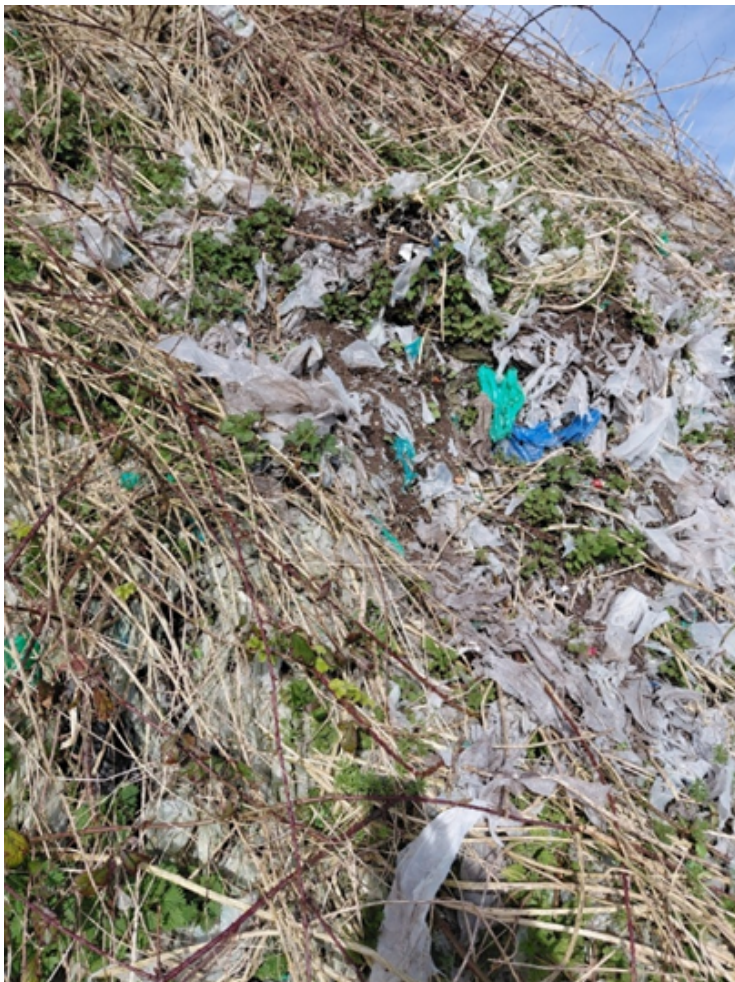
Figure 7 Photo showing degraded quality of plastic and growth coming out of plastics, suggesting has been stockpiled for a substantial period of time.
