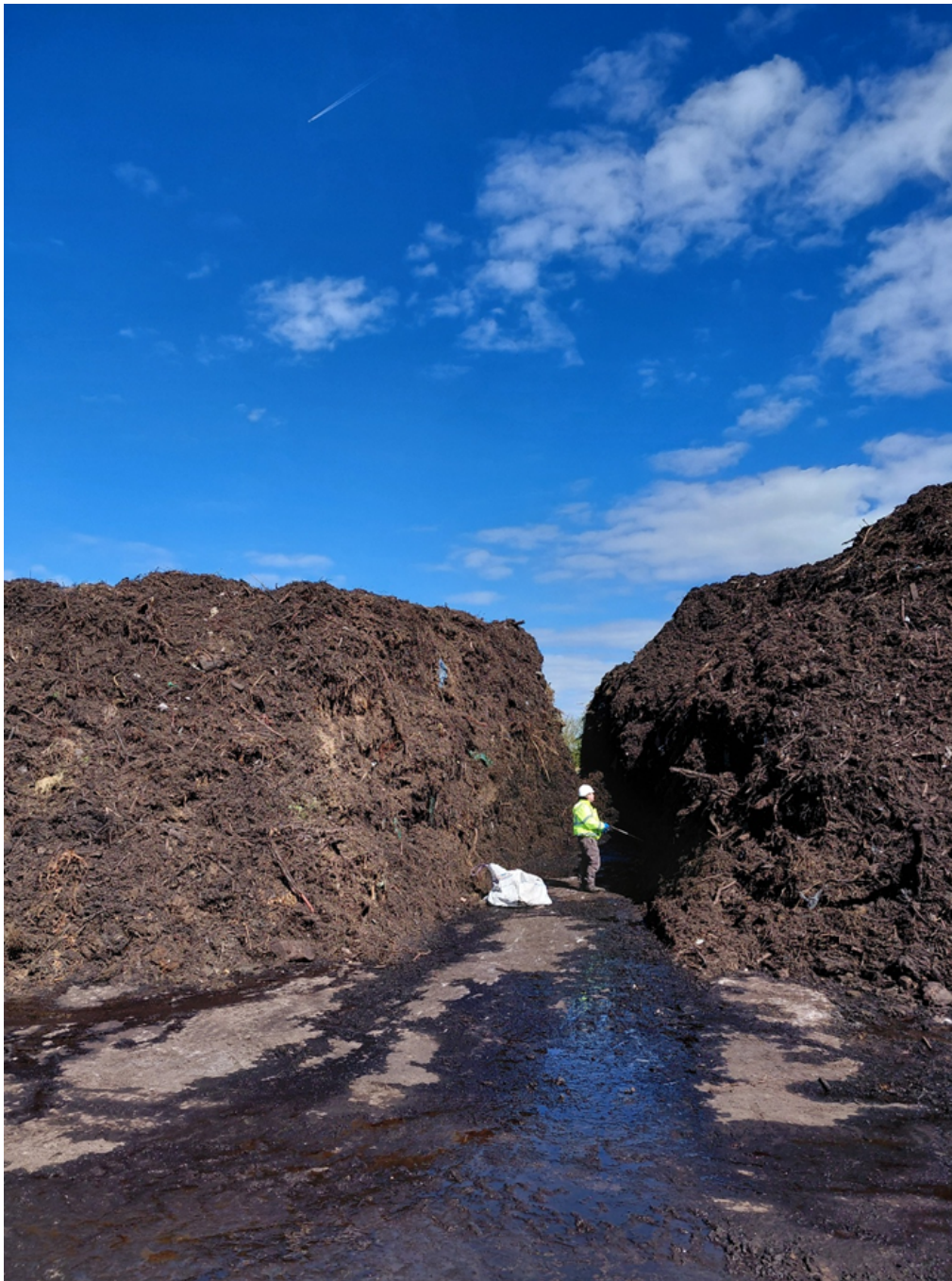
Figure 1 - Legacy green waste stock pile, showing poorly formed fire breaks
