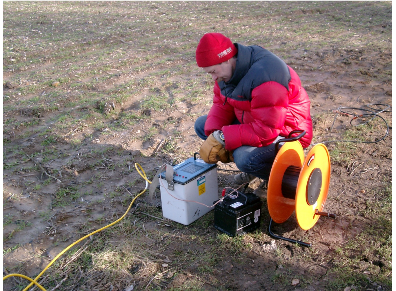
Figure 4. ERT survey. A: cables and electrodes positioned in ground. B: Controller and battery connected to cables.
