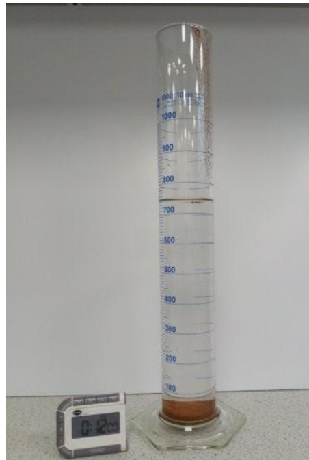
Treated sample – 12-mins settlement
