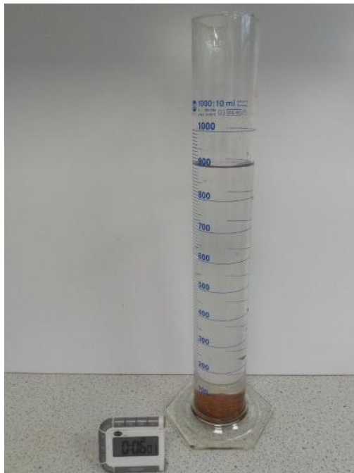
Treated sample – 6-mins settlement
