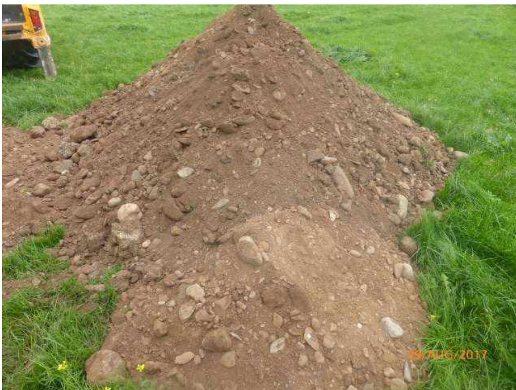
Photo 2 – Arising's from Trial Pit 01
