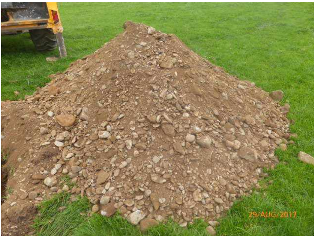
Photo 22 – Arising's from Trial Pit 11
