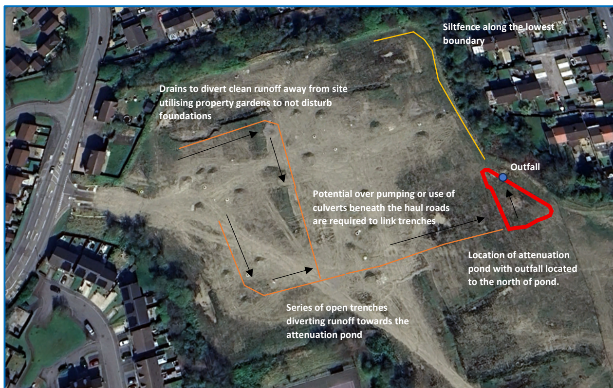
Figure 11: Phase 1A – Pollution Control Measures (ditches to feed Pond E will be moved and updated as the development progresses).
