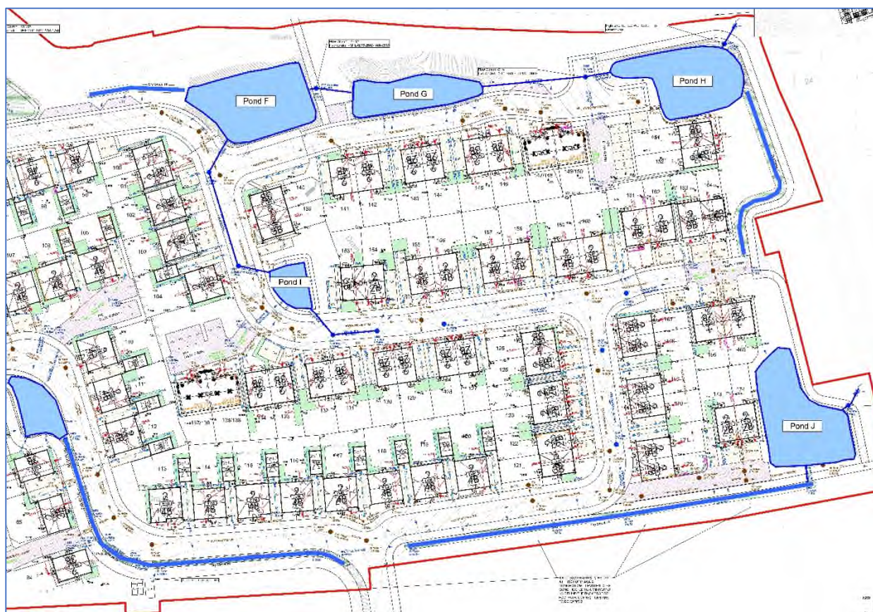
Figure 15 – Phase 1B Construction Runoff Mitigation.
