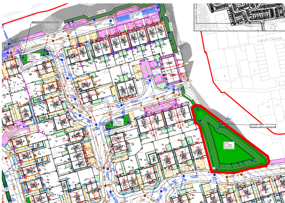
Figure 10: Location of Pond E - to be used as Construction Runoff Attenuation Pond.
