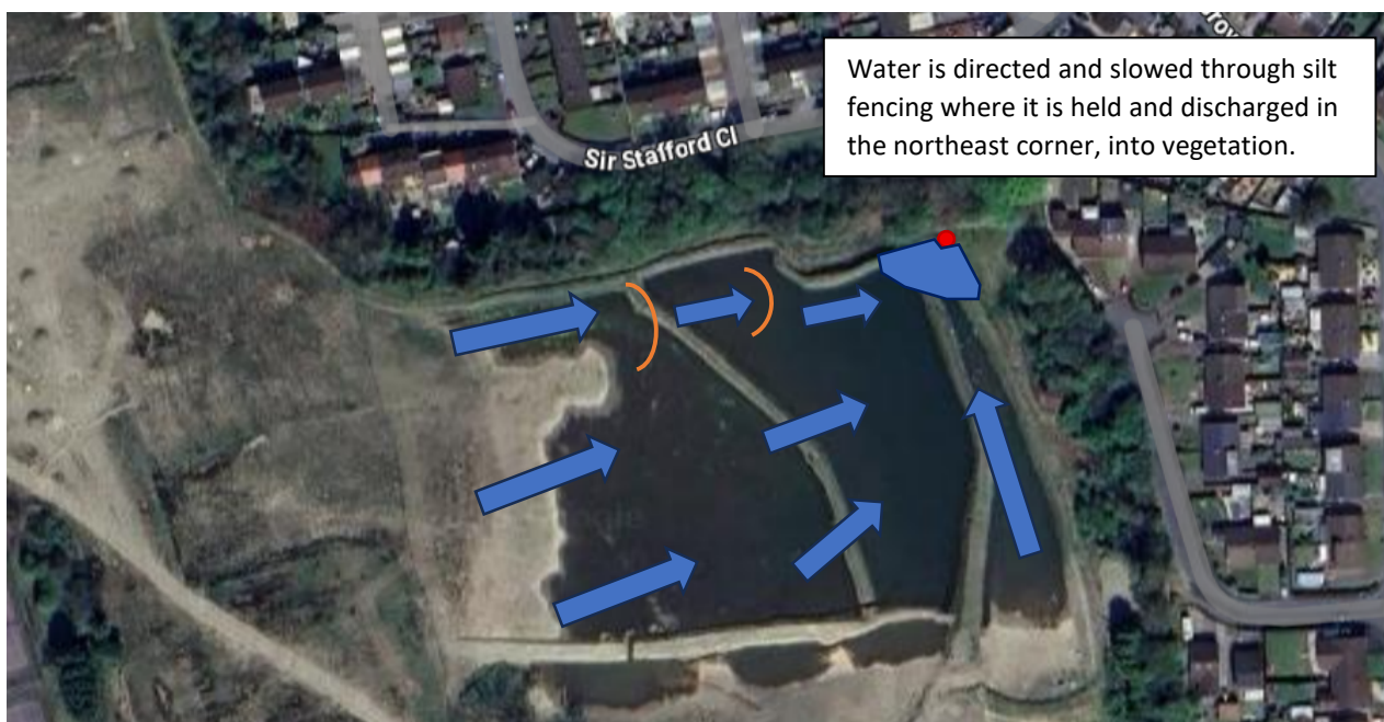
Figure 8 - Existing runoff controls and direction of surface runoff flow
